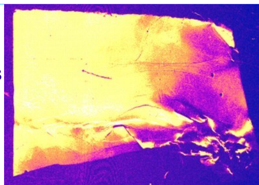
CdZnTe wafer (111) and its X-ray tomography image
